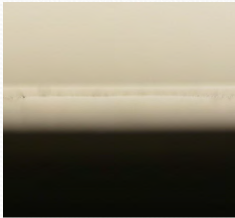
Right after 50W, 60s plasma cleaning. Water contact angle is too low to be measured.
