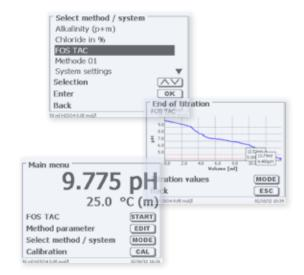
TAC = ml  $H_2SO_4$  to pH 5.0 × 250 FOS = (ml  $H_2SO_4$  from pH 5.0 to pH 4.4 × 1.66 - 0.15) × 500
