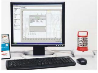
Applications: implementing a comprehensive routine control of steam sterilizers by means of the alternative Bowie&Dick-Test
