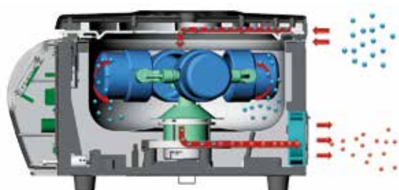
Unique air flow structure for effective noise reduction and excellent cooling
