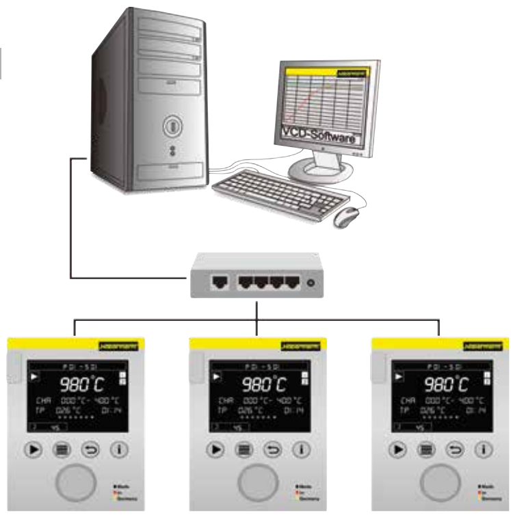
Example lay-out with 3 furnaces
